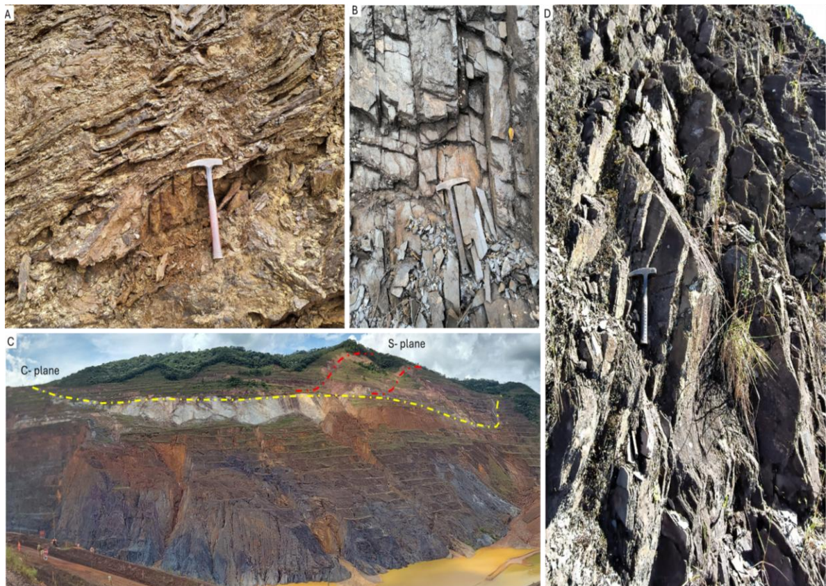
Figure 32: A) Schistosity in dolomitic itabirite of the Gandarela Formation. B) Spaced cleavage observed in compact itabirites of the Cauê Formation. C) Shear zones along the northern pit wall act as weak planes. D) Conjugate fracture patterns in siliceous itabirite from Cauê Formation.
