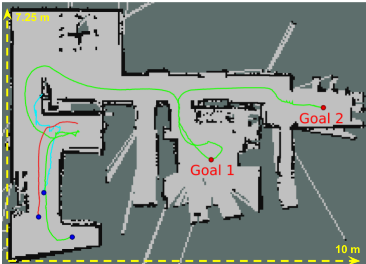
Figure 33 – Sim-to-real results of the experiments using our proposed navigation police (green path), using SAC from Hu et al. [2020a] (cyan path), and using PFC (red path) for the robot navigating in an office-like environment. The green line represents the robot's path from the starting point (blue) to the goal points (red). The grey area is the free space on the map, black points are obstacles, and dark green is the unknown area or places to be discovered.
