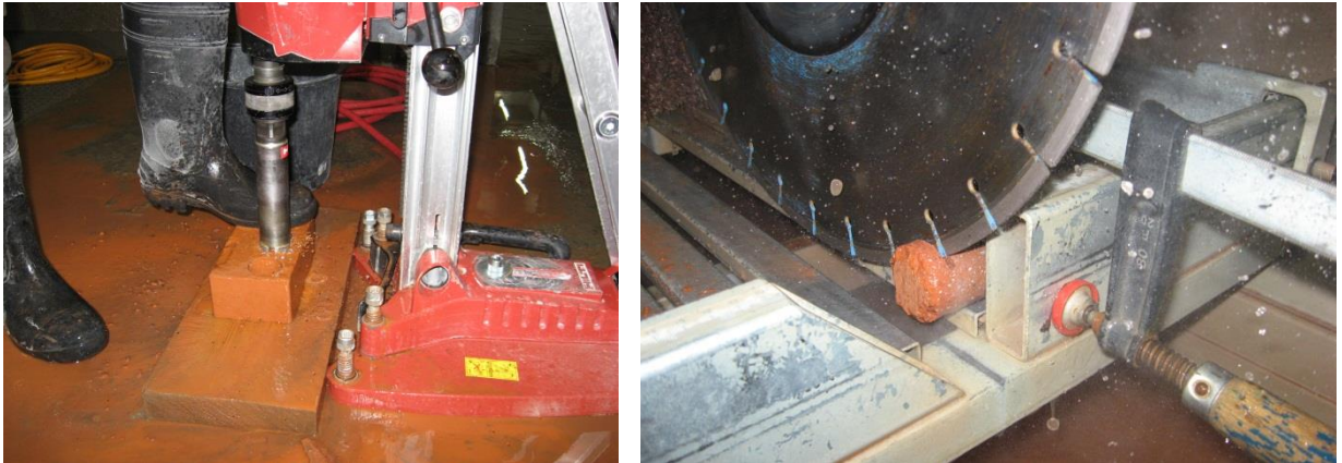
Figure 2.8 - Preparation of the ceramic brick geometry, cutting in cylindrical form (left) and cutting the body for the specified height (right)
