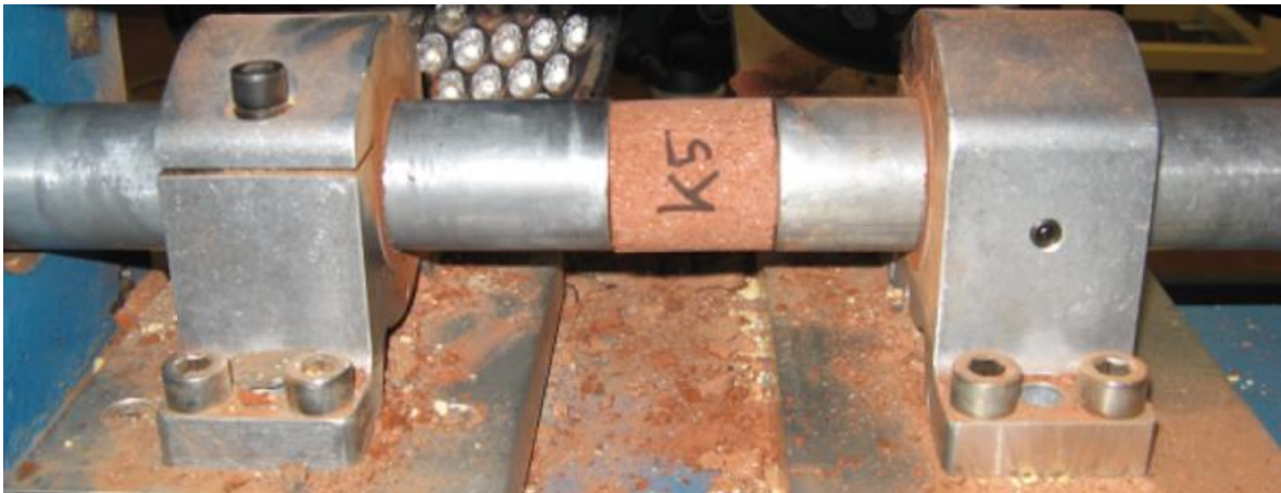
Figure 2.19 – Dynamic compression test conducted in Split-Hopkinson-Bars
