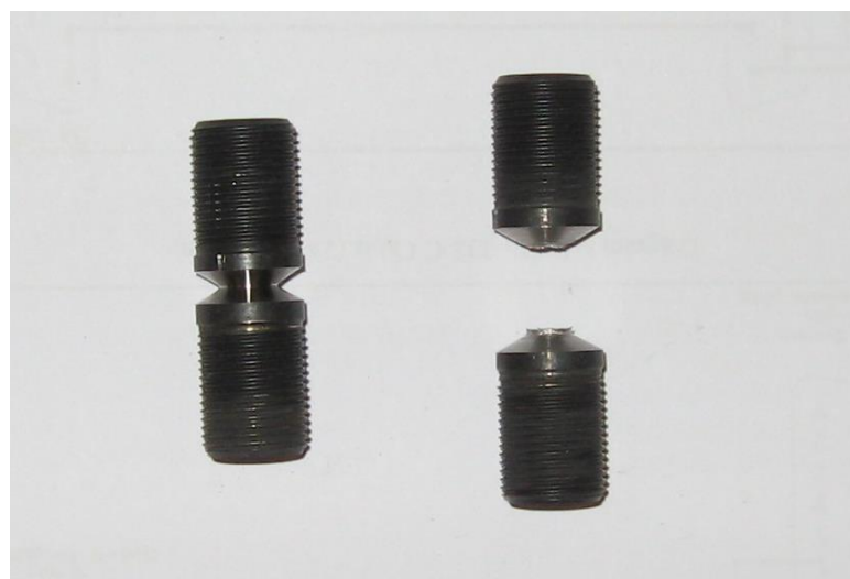
Figure 2.17 - Used impact system for the Split-Hopkinson-Bar
