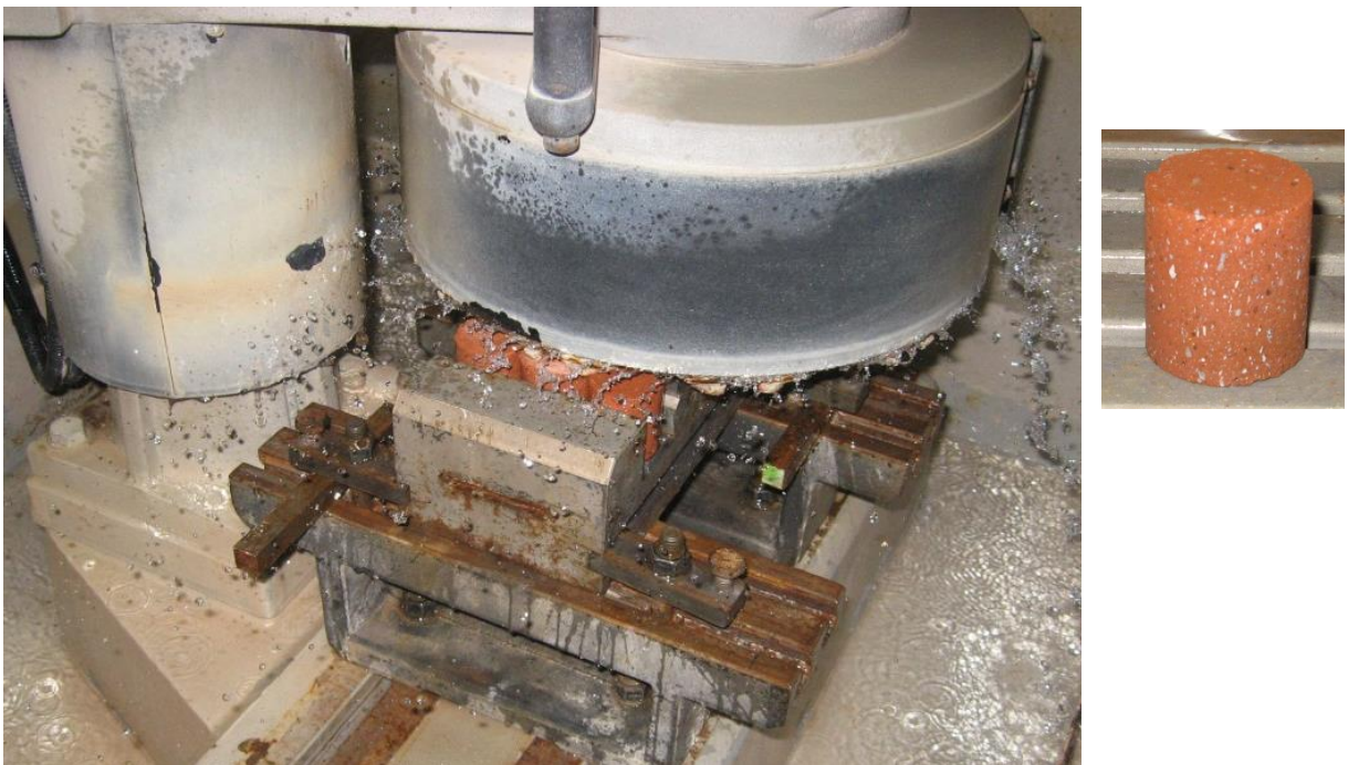
Figure 2.9 - Polishing the bottom and top faces (left) and cylindrical ceramic specimen after polishing (right)
