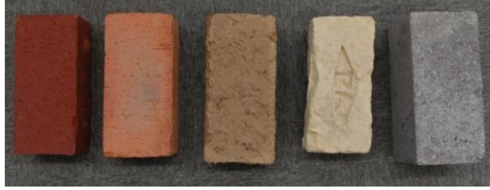
Figure 1.11 - Examined bricks (left to right): clinker, ceramic, German clay, Afghan clay and concrete
