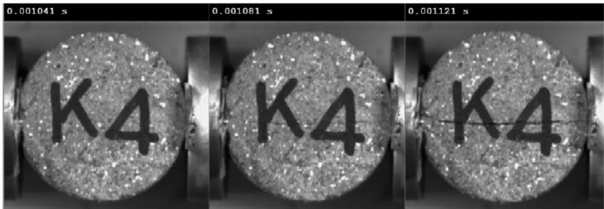
Figure 2.18 - Crack propagation during indirect dynamic tensile test, Brazilian test
