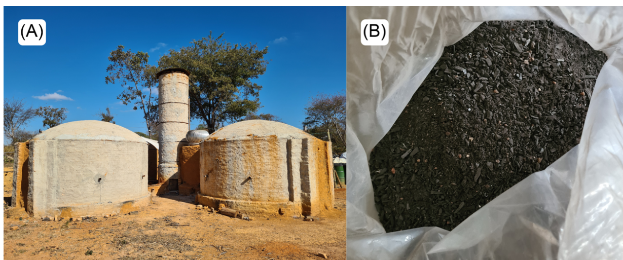
Figure S1. (A) Kiln-furnace system; (B) Charcoal fines (biochar) from pyrolysis at 450 °C.
