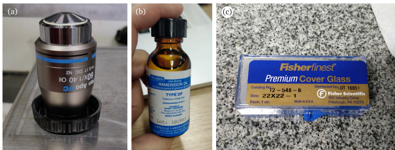
FIGURE B.1: (a) The microscope objective used in the system is a Nikon Plan Apochromat VC Objective, 60x, 1.4 NA, Oil. (b) The immersion oil used is a cargill #16242 or #16482. (c) The microscopy coverslips are from Fisherfinest Premium cover glass model #12-548B, measuring 22 × 22 mm and with an approximate thickness of 0.13 to 0.17 mm.
