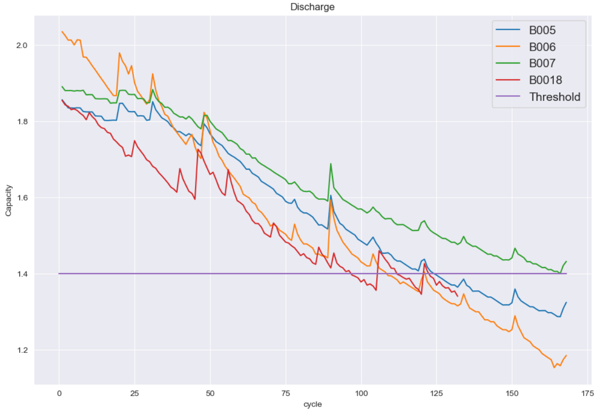
Figure 28 – Battery capacity over time (cycles)
