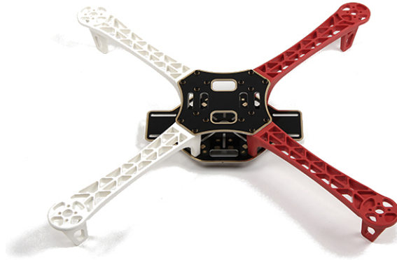
Figure 3.1: HK-450 Quadrotor frame. The DJI-450 frame and its derivatives are very commonly used, which makes parts availability and compatibility much easier. The 450 stands from the diagonal distance between motor shafts, this is a medium frame.
