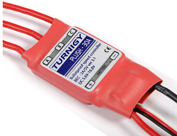
Figure 3.4: Turnigy Plush 30A Electronic Speed Controller. This model has different components dependent on its manufacture date. Our features SiLabs microcontrollers and both NPN and PNP transistors. Like our motors, these ESCs can work with both, 3 cells and 4 cells batteries.
