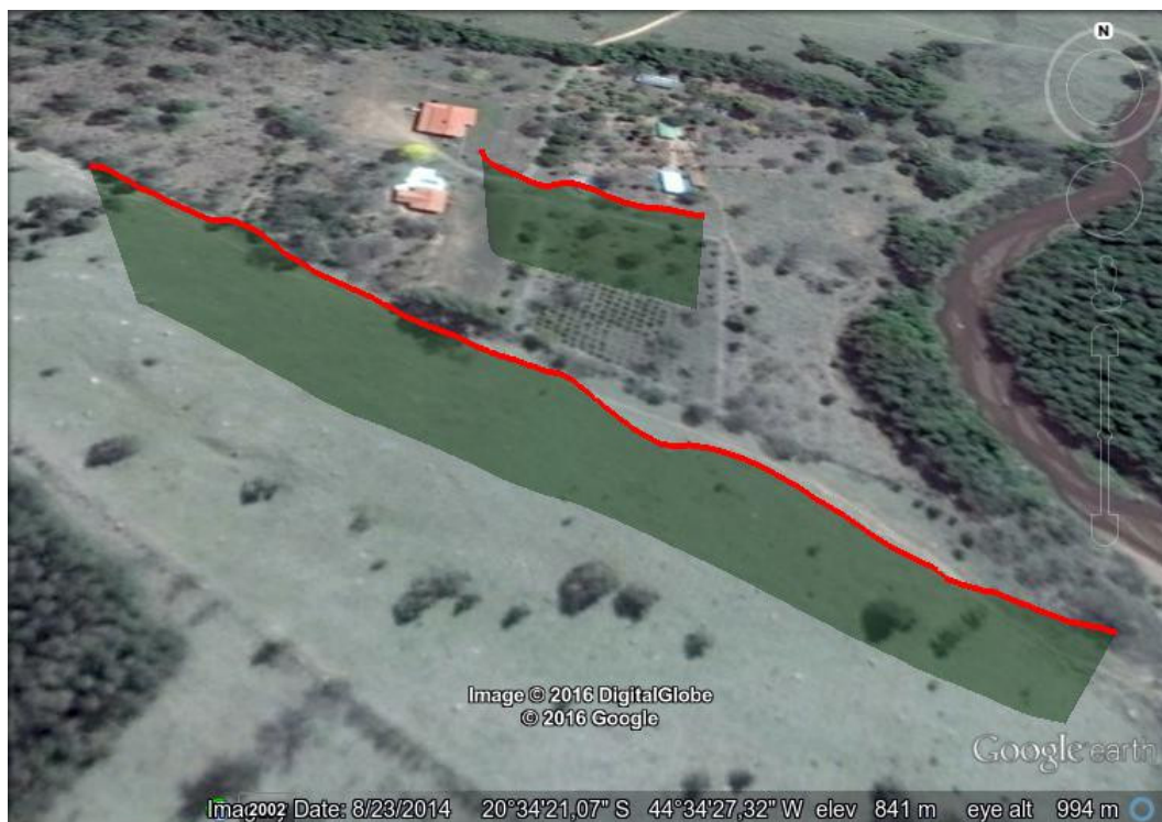
Figure 5.10: Mountain flight path from GPS data of the telemetry logs. This image is from a perspective view, where the red lines represent the flight paths of the two areas of interest and the green shade the projection of this flight path on earth's surface.
