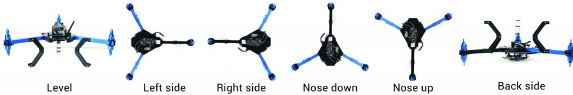
Figure A.14: Accelerometer calibration positions for an hexarotor.
