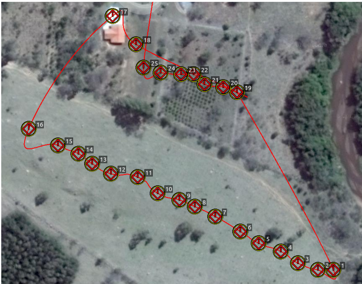
Figure 5.8: Mountain flight plan. It shows the flight plan for the mountain video sequence, the first slope is between waypoints 1 and 16, and the second between waypoints 19 and 25.
