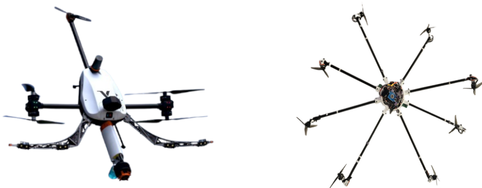
Figure 1.1: One application of our strategy is the control of omnidirectional drones, like (left) a Voliro drone (image taken from https://voliro.com ) and (right) the design from Hamandi et al. (2024) . Since they accept arbitrary 6 DoF twists, our methodology can be used to control them to track arbitrary differentiable paths in SE(3) .
