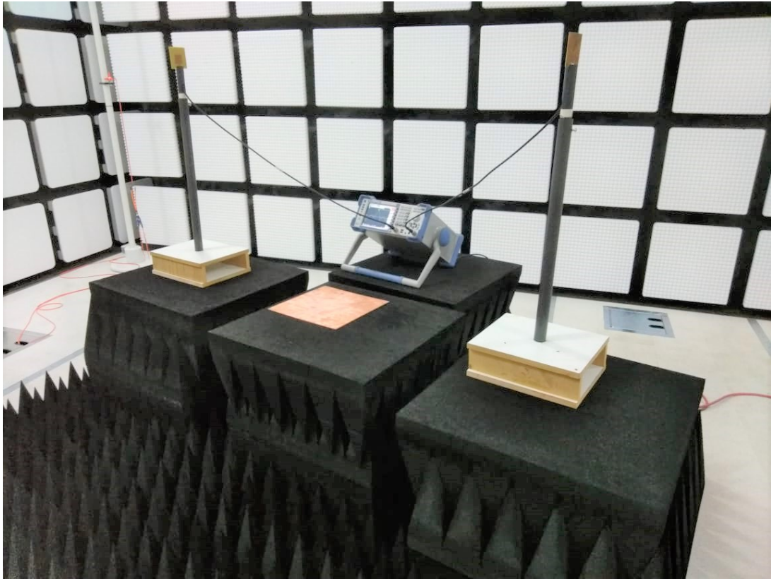
Figure 3.7 – Measurements in Cha1 using a copper plate as reflector to introduce multipath.
