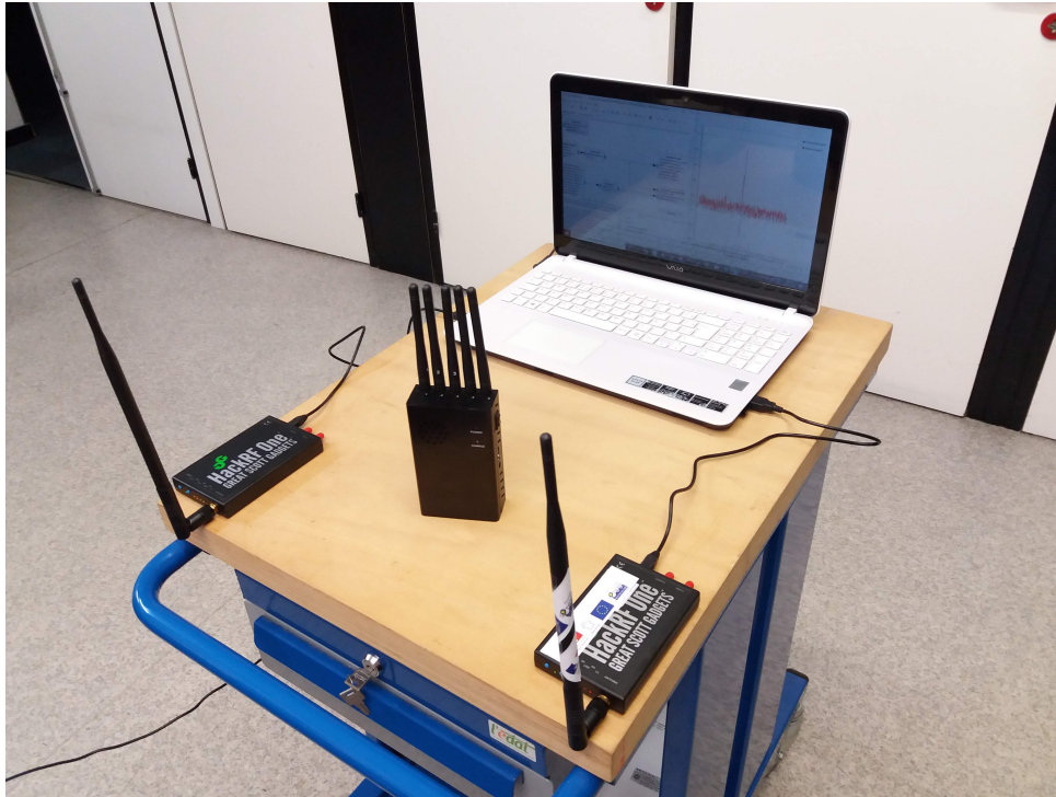
Figure B.1 – SDR-based test setup used to emulate a GSM-R communication link corrupted by IEMI. Equipment: a computer with a signal processing toolbox, a transmitting/receiving set and a jammer.
