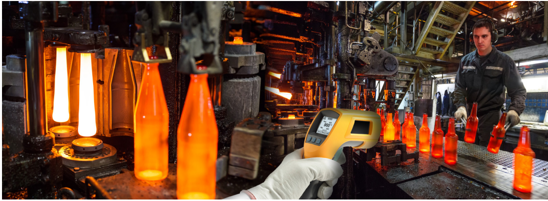
Figure A.1: Use of non-contact temperature-measurement device on industrial facility (glass bottle manufacturing). Edited (by the author) from the original photographs in [74].
