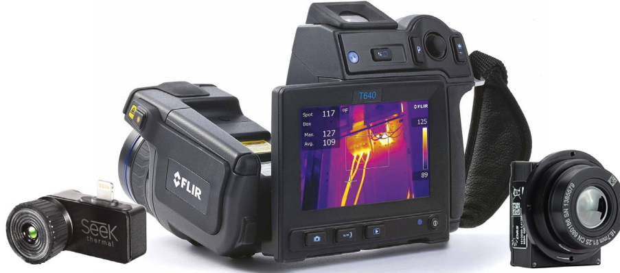
Figure A.16: Different thermal camera models and features. (Left) Portable thermal camera detects temperatures from -40 to 330\text{ }^{\circ}\text{C} with a 206\times 156 resolution, available from Seek Thermal [110]. (Center) Camera with uncooled microbolometer, 640\times 480 resolution, and 0.02\text{ }^{\circ}\text{C} sensitivity at 30\text{ }^{\circ}\text{C} , reaching temperatures up to 2000\text{ }^{\circ}\text{C} , from FLIR [108]. (Right) Uncooled LWIR camera with vanadium oxide detector and 640\times 480 resolution, from DRS Technologies [111].
