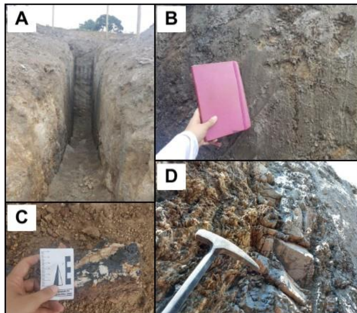
Fig. 3. Graphite schist sampling site. (A) Front view of trench; (B) Place where samples LR44A and LR44B were collected; (C) Sample LR44C, collected from quartz vein with presence of todorokite and manganite; (D) Quartz vein where sample LR44C was collected.
