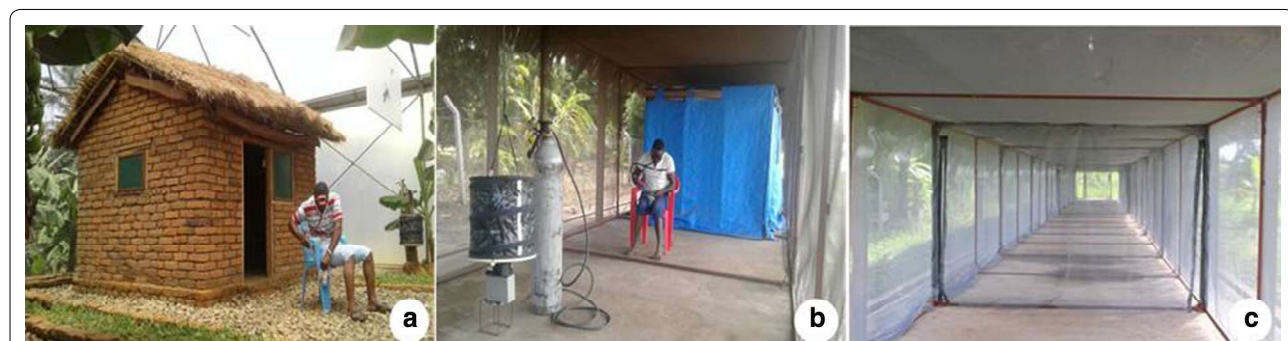
Fig. 1 Pictorial illustration of the semi-field chambers and the mosquito tunnel. The semi-field chambers were used to evaluate the different configuration of push-and-pull subunits (a). The 110 m long mosquito tunnel was used to evaluate the optimal distances between the eave-ribbons wrapped along the eave-space of the hut (blue structure inside the chamber) and the odour-baited BG-Malaria trap (b). A section of the empty tunnel is also shown (c). Adult male volunteers sat in the peri-domestic space of each of the huts and collected mosquitoes attempting to bite them between 1800 and 2200 h, before going indoors to sleep under intact bed nets. CDC-light traps were used to catch mosquitoes attempting to bite the sleeper between 2200 and 0630 h the next morning
