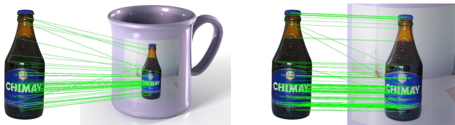
Figure 1.1. Keypoints being applied to object identification within different images. Each line marks the correspondence between keypoints from both images. Figure taken from Rusu [2010]
