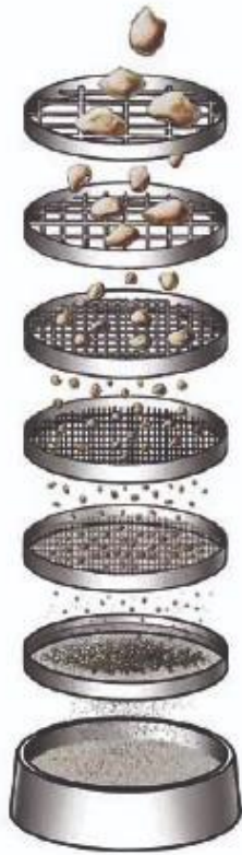
Figure 5-7: Example of functionality of the granulometric screen procedure.
