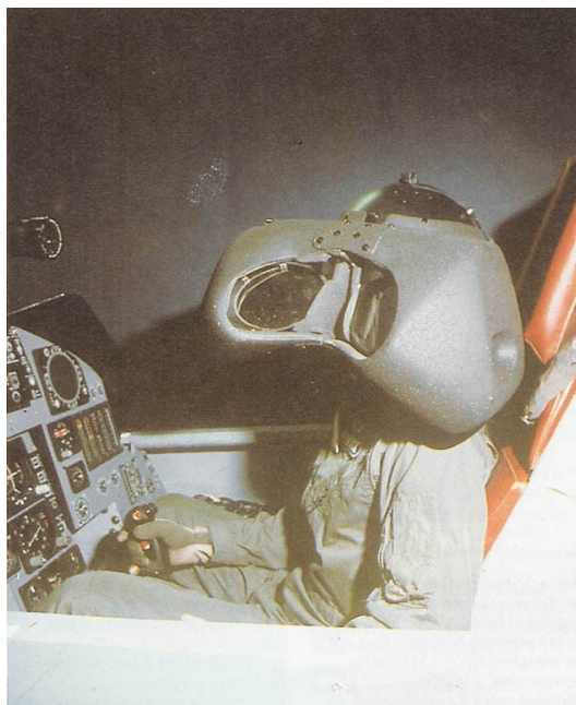
Figura 17 - Visually Coupled Airborne Systems Simulator, precursor do Super Cockpit 87 .
