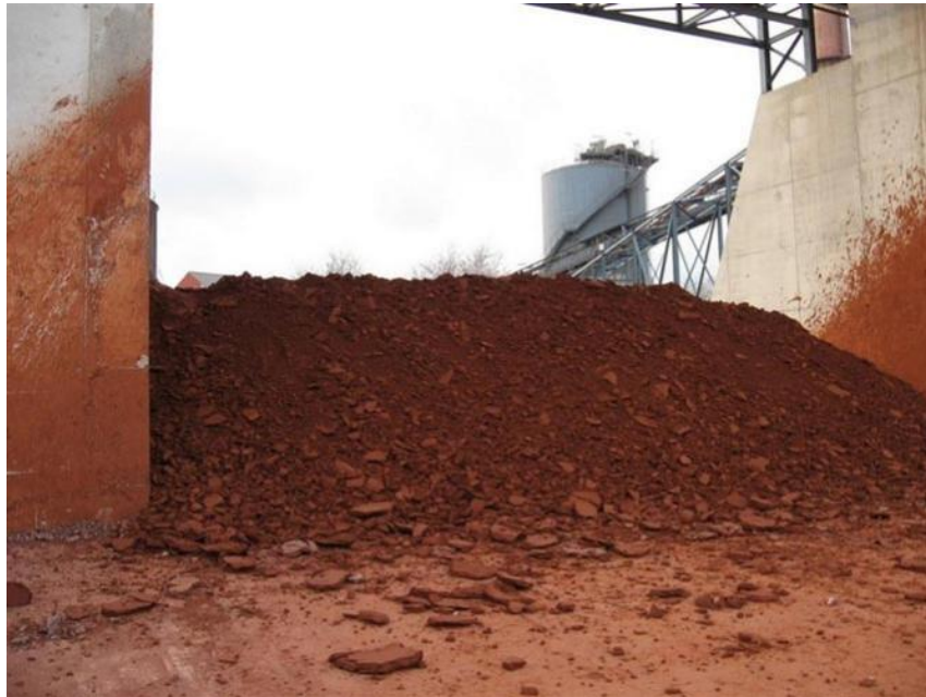
FIGURA 1.1 – Resíduo de alumina após a descarga do filtro prensa ( http://www.diemmefiltration.com/en/red-mud-filtration.html )
