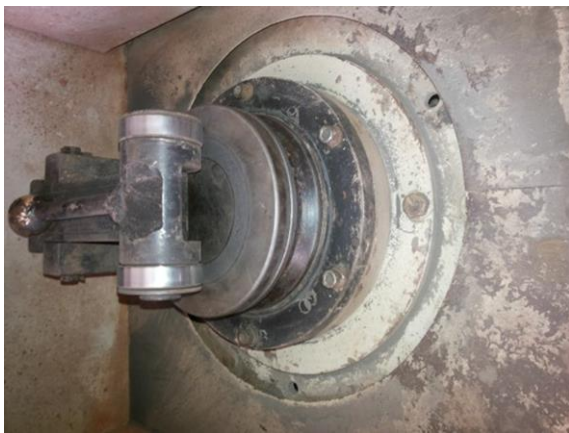
Figure 1. Apparatus used to grind titanium chips into fine particles.
