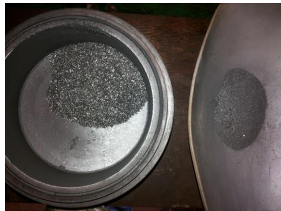
Figure 2. Aspects of the chip after the process of grinding (left) and classified in a 400\mu\text{m} vibrating screen (right).
