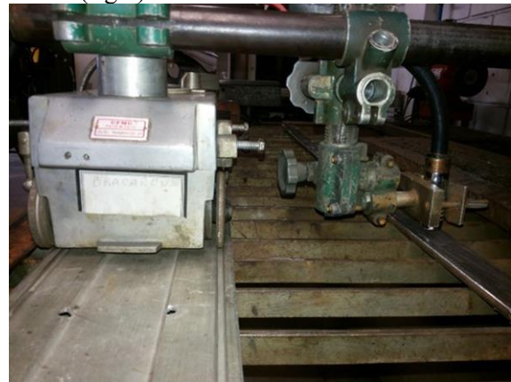
Figure 4. Welding scheme used to deposit the weld cladding on substrate.
