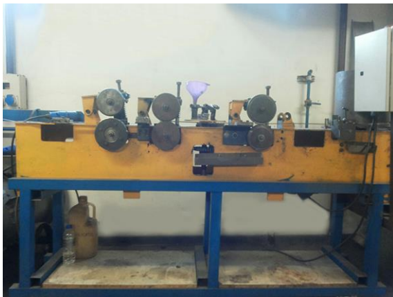
Figure 3. Experimental equipment of forming, filling and reduction of tubular wires.
