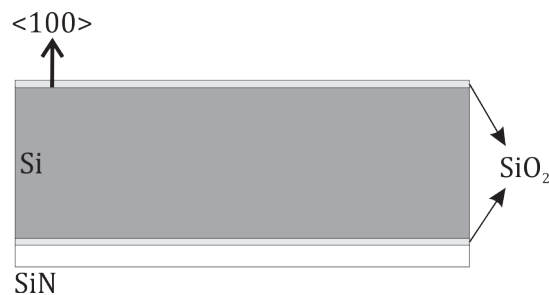
Figure 70 – Illustration of the silicon wafer used in the fabrication of the microlens array.
