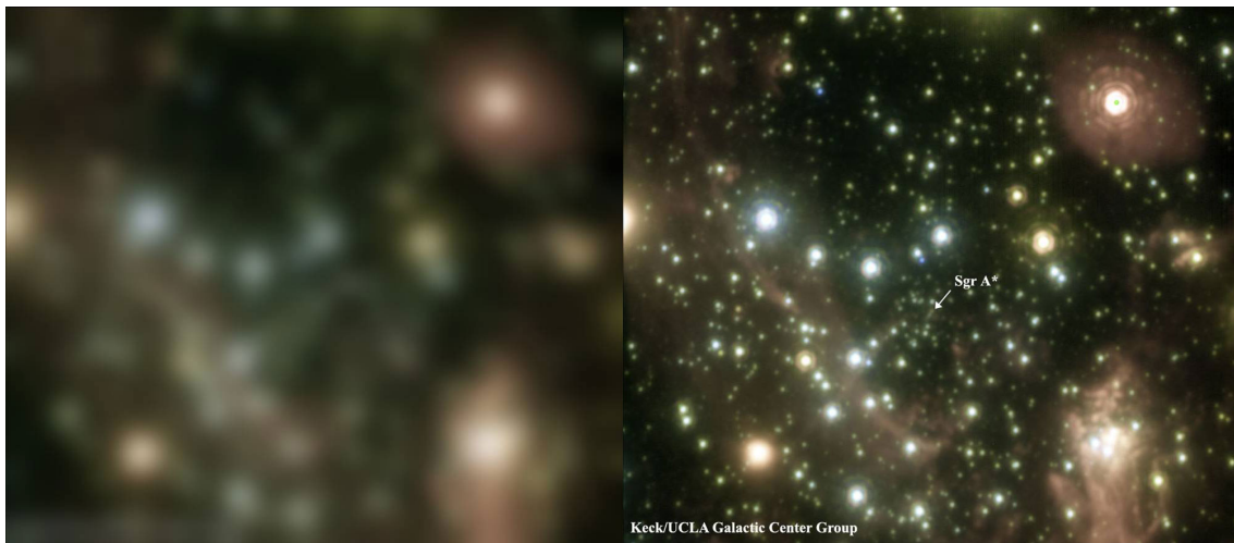
Figure 49 – Astronomical images taken with (right) and without (left) AO (KECK OBSERVATORY; UCLA GALACTIC CENTER GROUP, 2007/2008).
