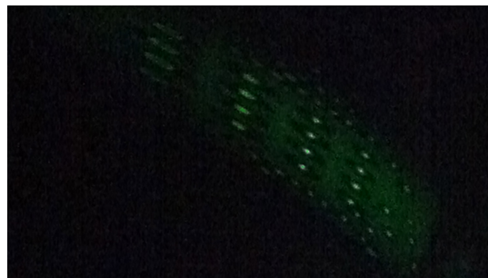
Figure 77 – Image generated by the 16-microlens rectangular array in the proximity of the focal plane.
