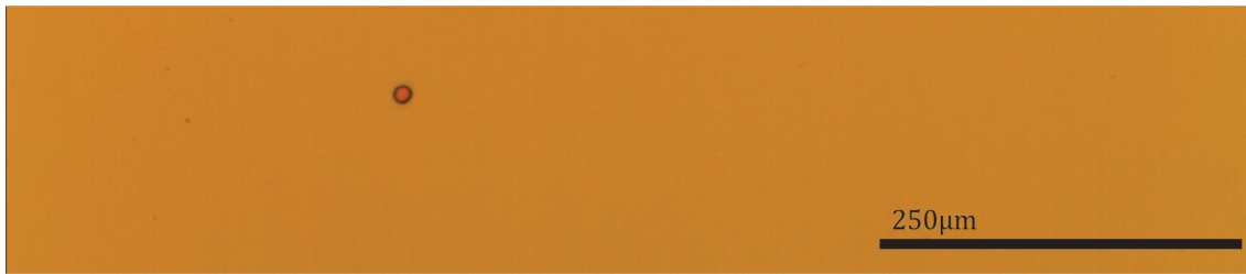
Figure 71 – Pattern transferred to the photoresist layer. The lateral dimension of the opening is about 10 μm.
