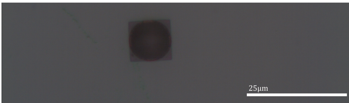
Figure 72 – Inverted pyramid formed after KOH etching.
