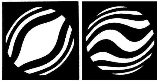
Figure 28 – Example of Ronchigrams. On left, the mirror introduces spherical aberration and on right, spherical aberration combined with astigmatism (MALACARA, 2007).
