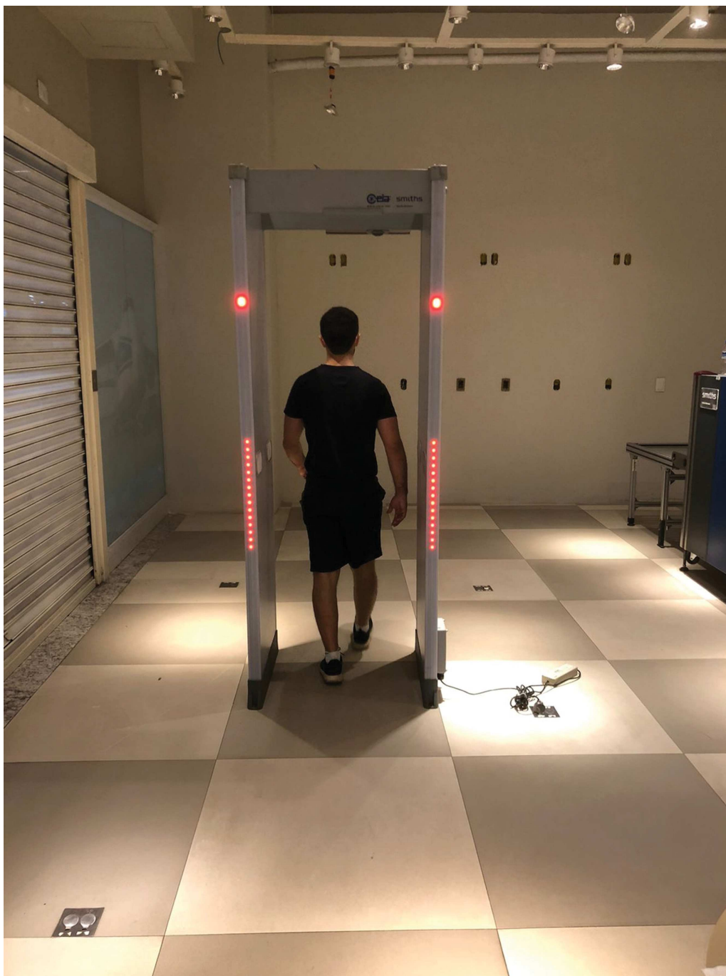
Fig. 2 Control test to certify appropriate functioning of the arch detector using cellphone in the pocket.
