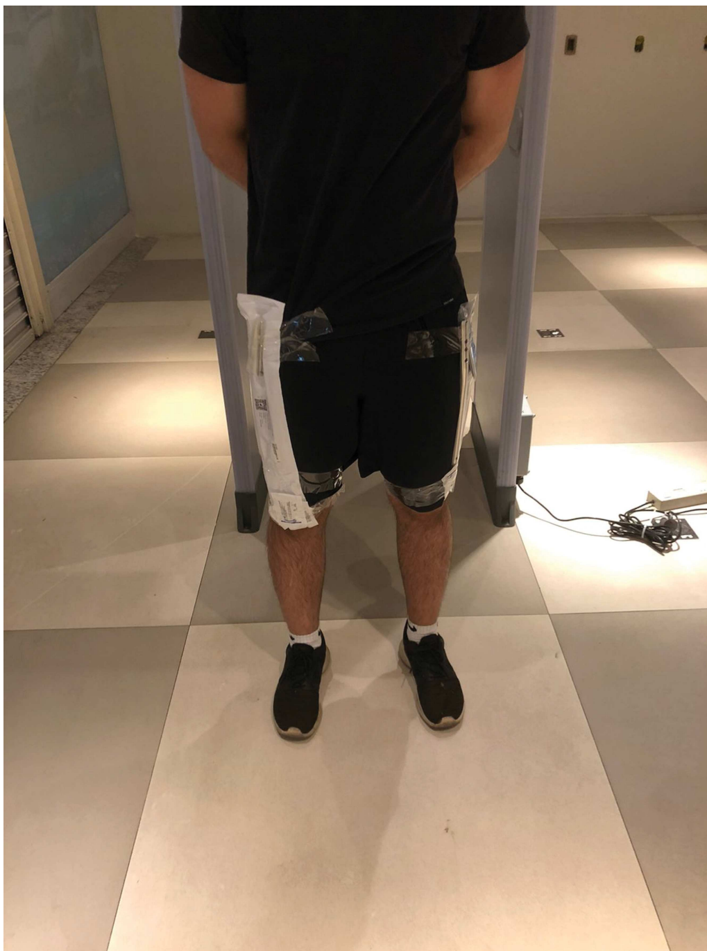
Fig. 4 Bilateral retrograde femoral nail strapped to the lateral surface of the thighs before testing.
