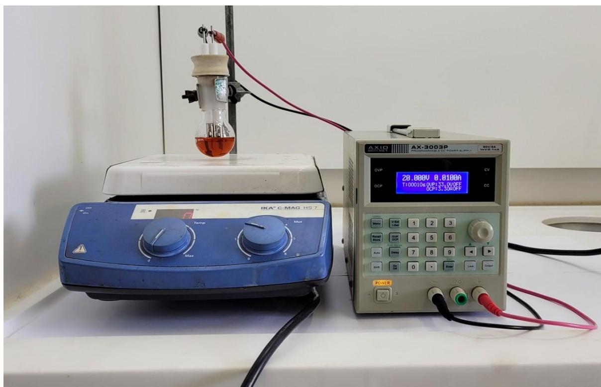
Figure 18: General apparatus for the electrosynthesis procedure.
