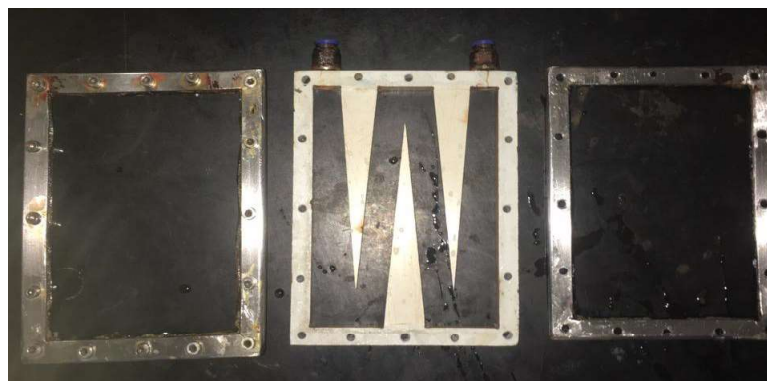
Figure A.5 - PMR module structure.
