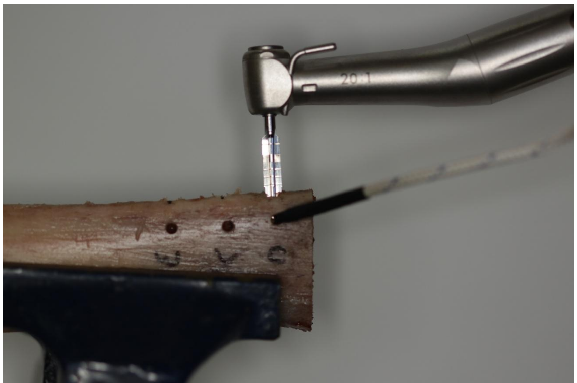
Figure 1 - Location of the thermocouple probe during osteotomy for each group
