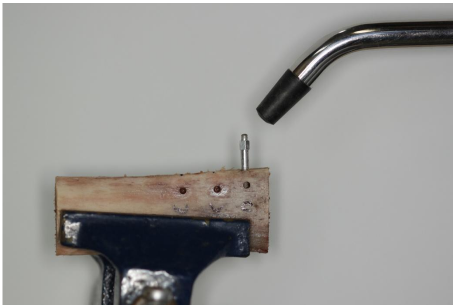
Figure 3 - Measurement of the resonance frequency of the implants
