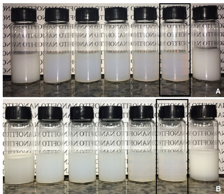
Figure 3. Set of emulsions prepared with H. suaveolens essential oil and the surfactants sorbitan monooleate/polysorbate 20 at different rates (from right to left: HLB of 10, 11, 12, 13, 14, 15, and 16.7). Highlighted is the rHLB of 15 since this is the HLB value of the mixture of surfactants that allowed the most stable nanoemulsion, with this being chosen for the bioassay. (A) Day 0 of preparation. (B) After 7 days of storage.
