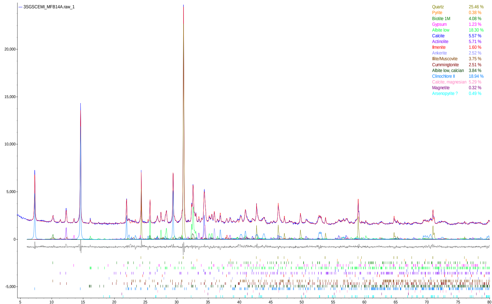
Rietveld refinement plot of sample SGS CEMI “MFB 14 A” (blue line - observed intensity at each step; red line - calculated pattern; solid grey line below – difference between observed and calculated intensities; vertical bars - positions of all Bragg reflections). Coloured lines are individual diffraction patterns of all phases.
