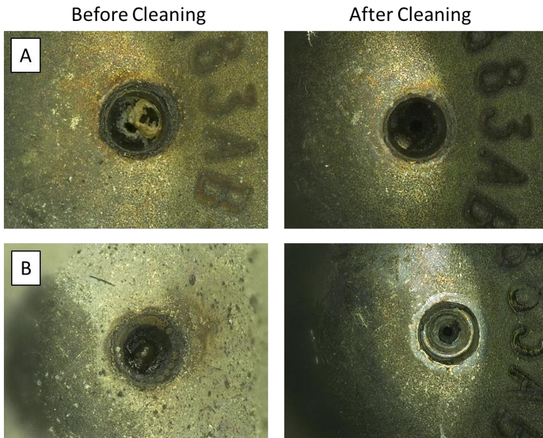
Figure 4.1 - Pre-chamber injector holes after A) 13-hour operation and B) 9-hour operation before and after ultrasonic bath
