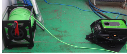
Figure 4.18. Experimental platform used to acquire sequence of images: an underwater vehicle Seabotix LBV300-5 equipped with a color camera.
