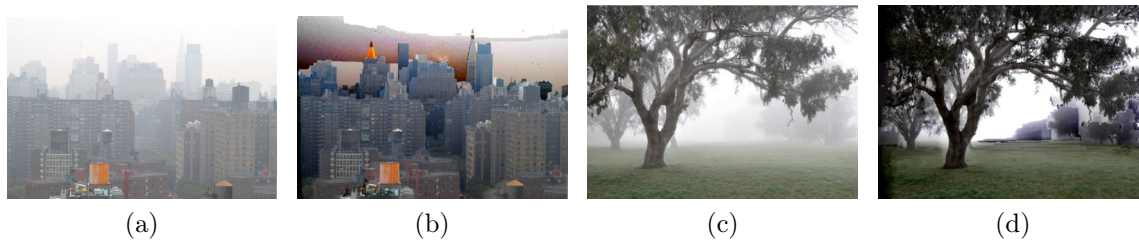
Figure 2.22. Example of image restoration results by Caraffa and Tarel [2012] in foggy scenes. (a,c) Original images, and (b,d) restored images. The results obtained present good improvement in near regions of the images, but some halos and color distortion are visible in farther regions.
