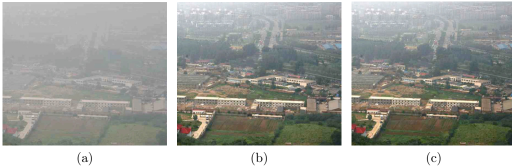
Figure 2.12. Image restoration results in a hazy scene obtained by Carr and Hartley [2009]. A foggy image (a) is restored the proposed method using monotonic model (b), and dark channel model [He et al., 2009] (c).
