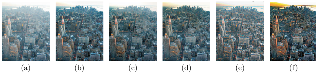
Figure 2.4. Image restoration results obtained by Ancuti et al. [2010] under hazy condition. (a) Original image, (b-e) restored using the method of Ancuti et al. [2010], Fattal [2008], He et al. [2009], Tarel and Hautière [2009], and Tan [2008], respectively.
