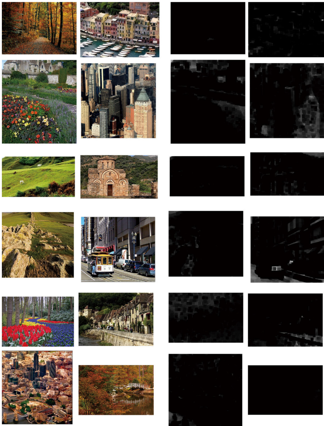
Figure 3.2. Dark channel prior [He, 2011]. Left: outdoor images acquired in non-participating media. Right: the corresponding dark channels. The dark channels are mostly dark. The images are resized so that the maximum of width and height is 500 pixels. Their dark channels are computed using a patch size 15 \times 15 .
