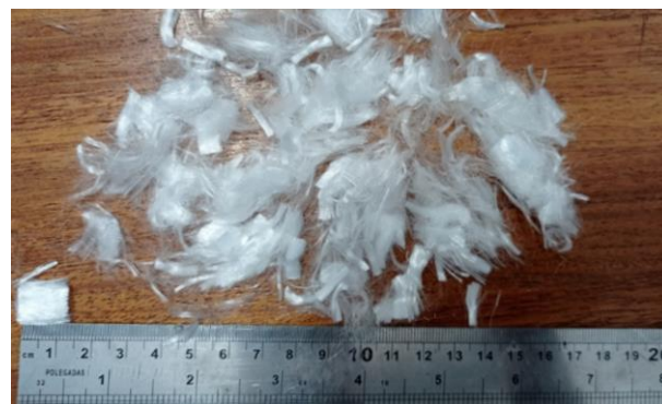
Figure 1. Polypropylene fibers supplied by Viapol.
