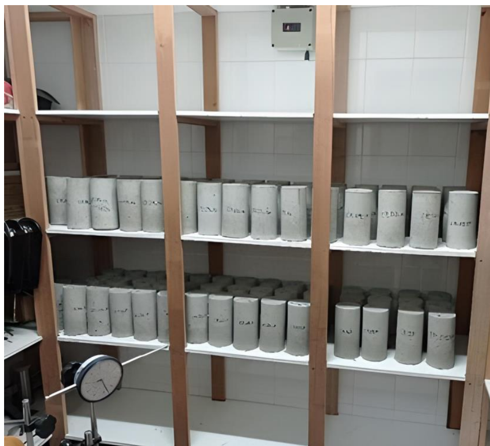
Figure 2. Mechanically treated ends' specimens stored in the climatized chamber.
