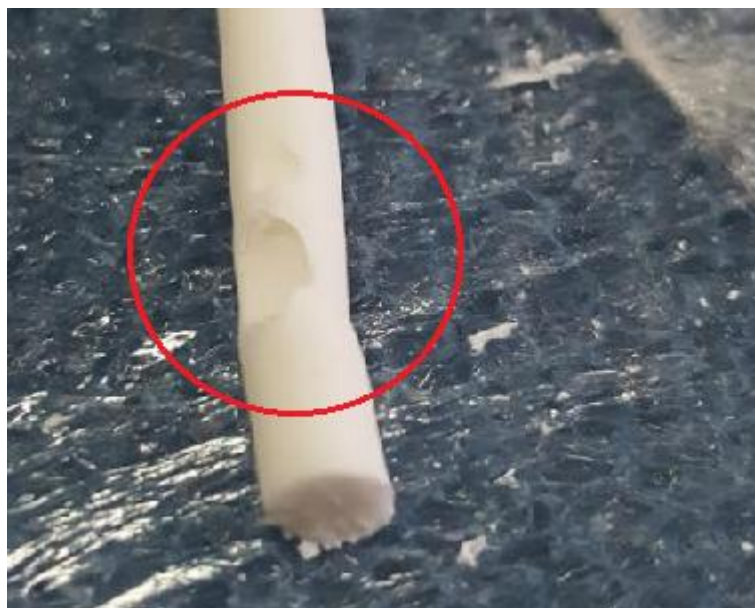
Figure 29: Appearance of defect on the surface of the green body extruder due to presence of bubbles inside the extruder.
