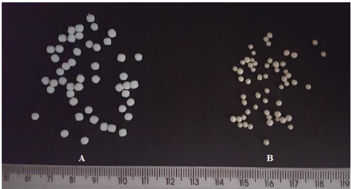
Figure 35: Photo of final fumed silica spherical granules prepared with 15 % of binder (A) and commercial zeolite granules.
