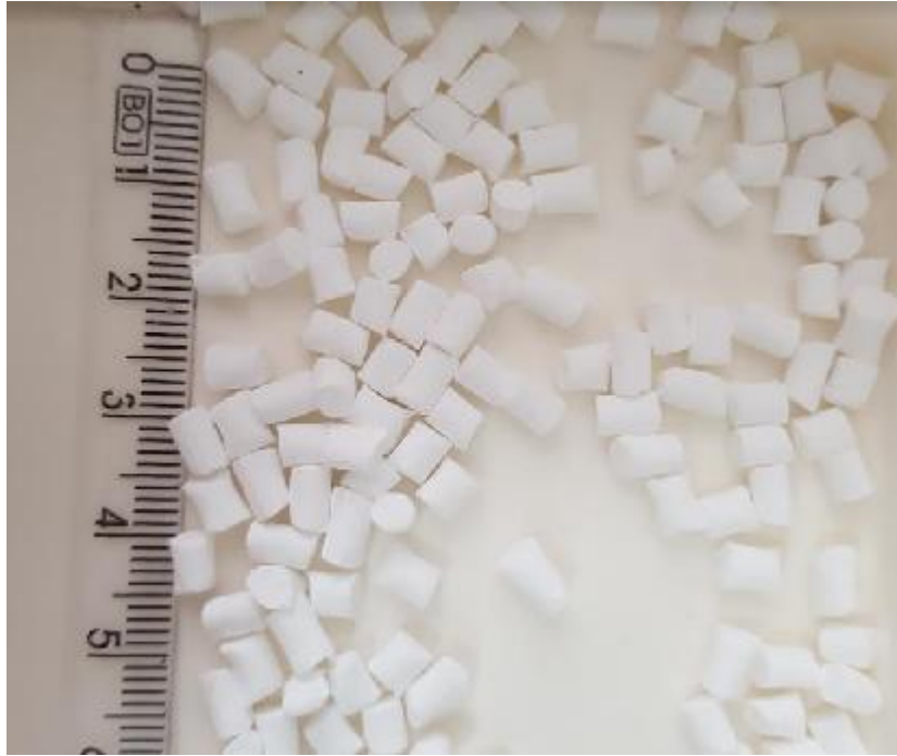
Figure 33: SBA-15 green body pellets prepared with 20 % of methocel.
