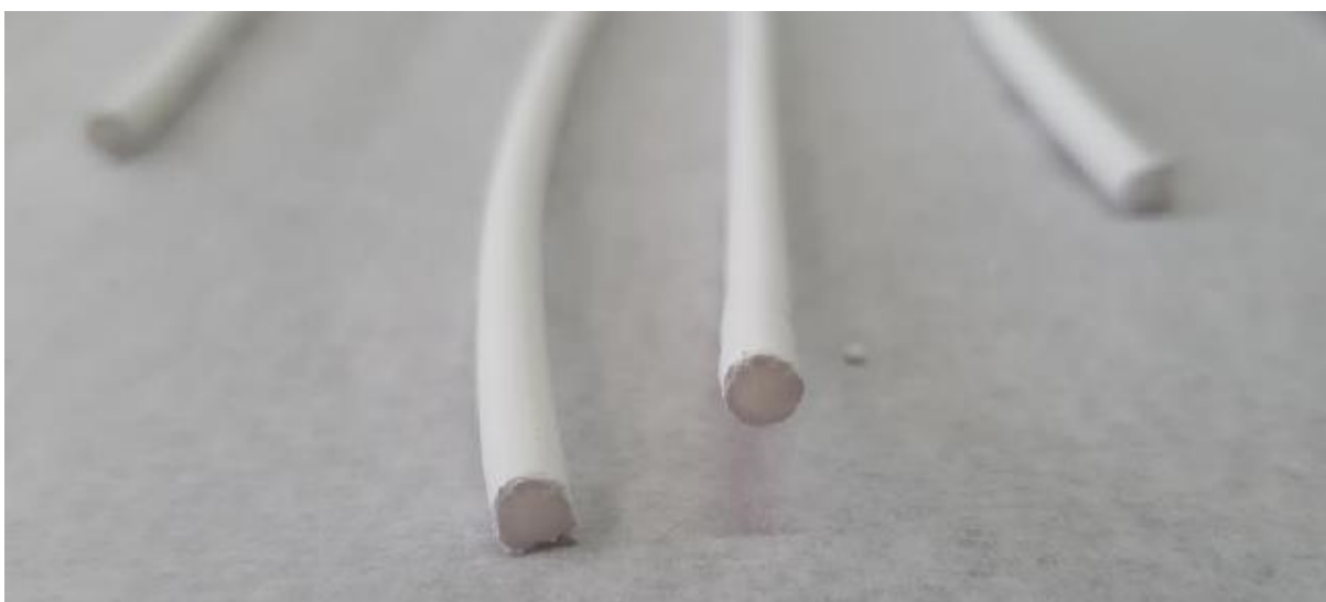
Figure 30: SBA-15 silica green body extrudates prepared with 20 % of methocel.
