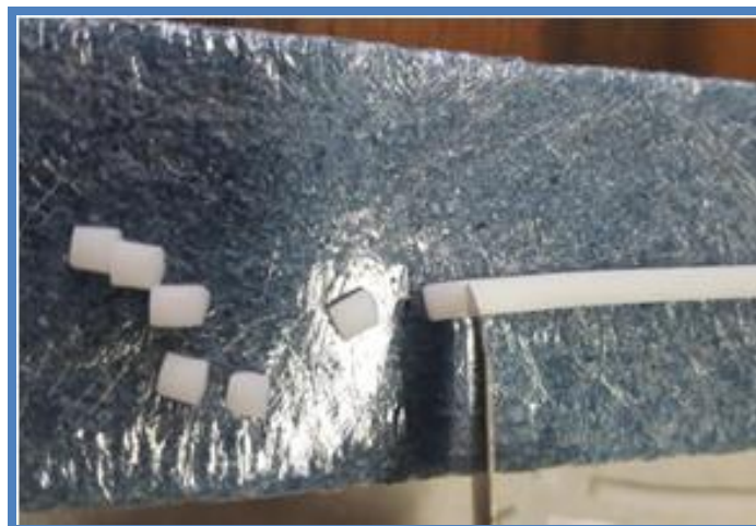
Figure 22: Wet extrudates in the sectioning procedure.
