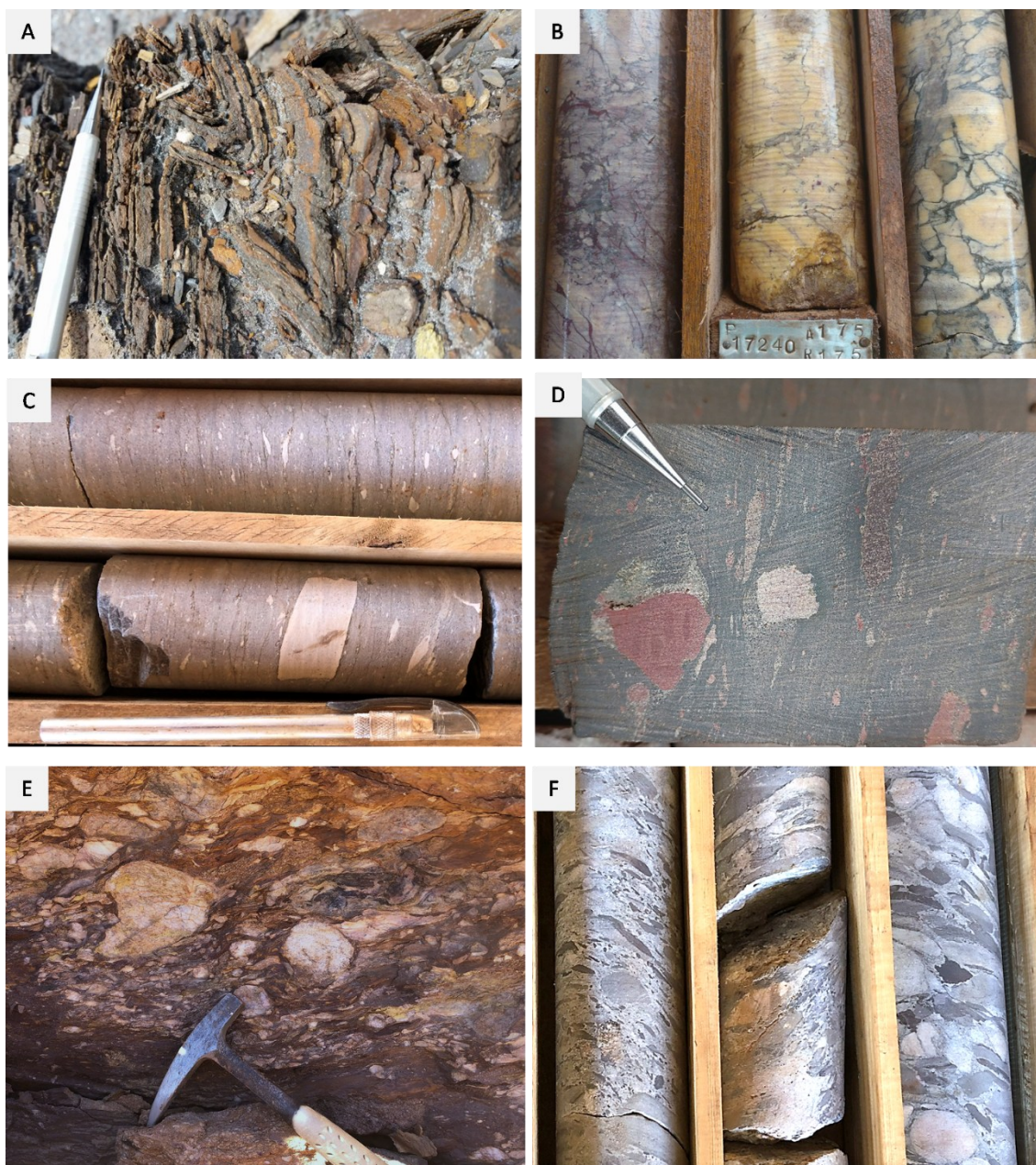
Figure 5: A - Folded quartz-itabirite layers from Cauê Formation; B - Drill core sample of brecciated dolostone; C –Metadiamictite with cobble of carbonates immersed in matrix ferruginous and carbonatic; D – Different shapes of carbonate clasts in metadiamictite; E - Matrix-supported metaconglomerate with diversified and deformed clasts associated with the Sabará Group; F - Drill core sample of metaconglomerates with clasts of quartzite and BIF from Itacolomi Group.
