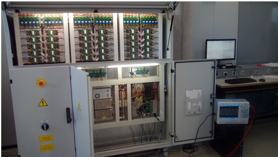
Figure 12. Modular Multilevel Converter prototype with five cells/arm.
