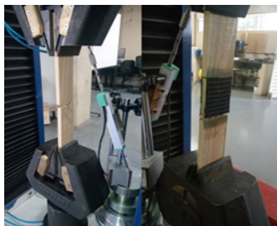
Figure 1: Tensile test for determination of tensile strength in the parallel direction in wood specimen of Pinus elliotti var. elliotti partially cracked.
