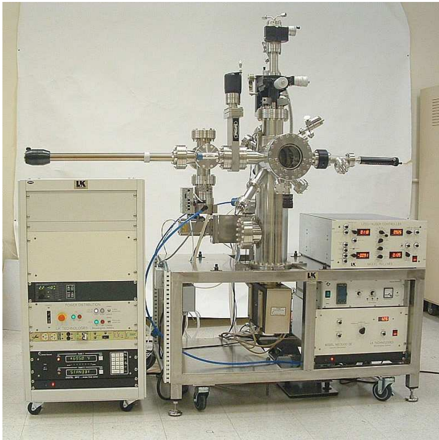
Figura 2.2: Aparato experimental LEED. [2]
