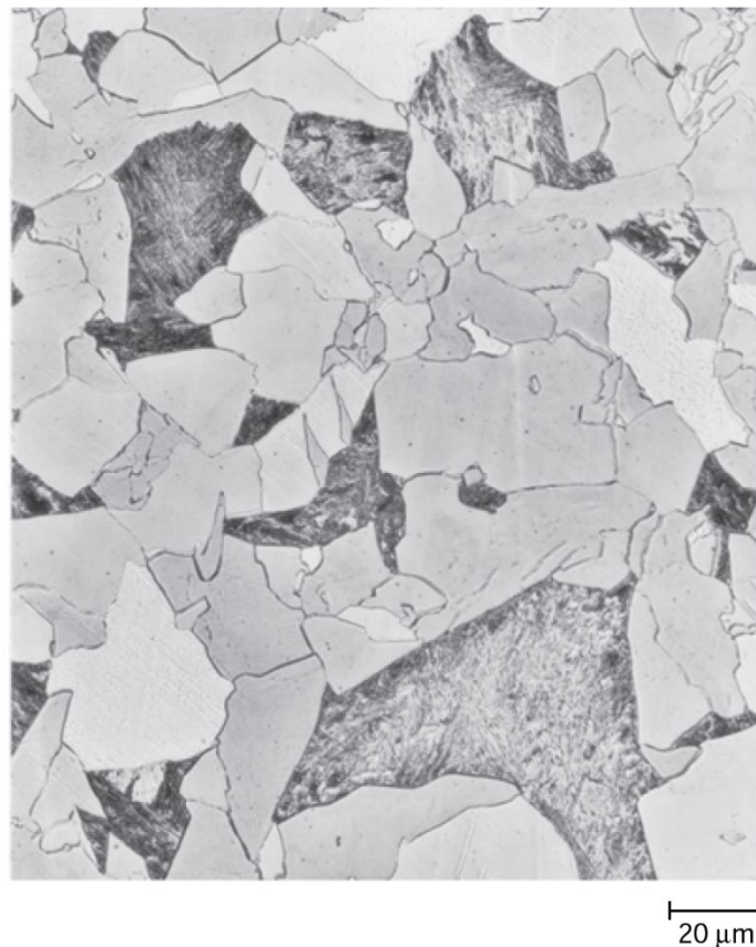
Figure 3.8 - Polygonal ferrite (light structure) formed in HSLA-80 steel isothermally transformed at 675 °C for 500 s [22] .
