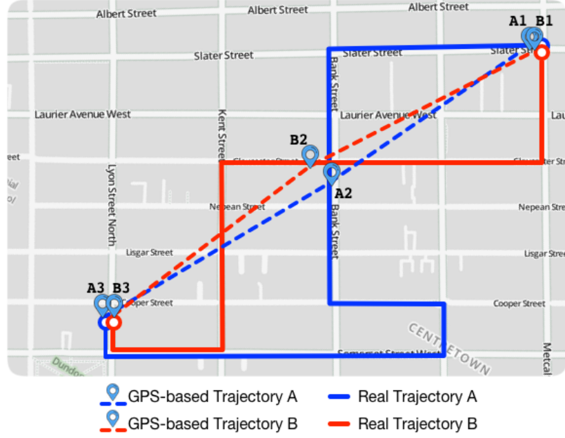
Figure 2.1: Two different GPS-based trajectories that look similar because of the gaps in the data.
