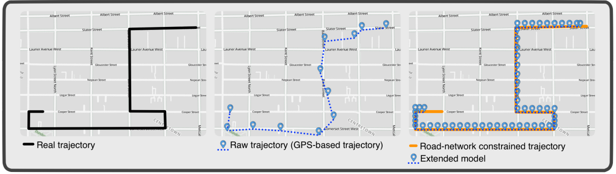
Figure 8.1: The extraction of an extended road-network constrained trajectory from a GPS-based trajectory.
