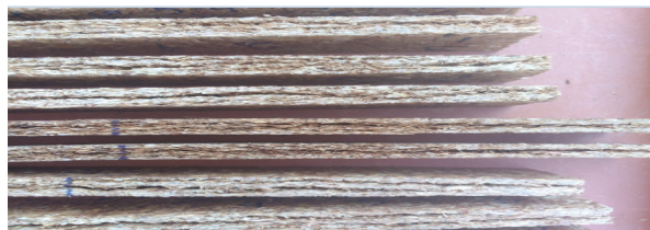
Fig. 1: Delamination panels produced according to Treatments 3 and 4.
