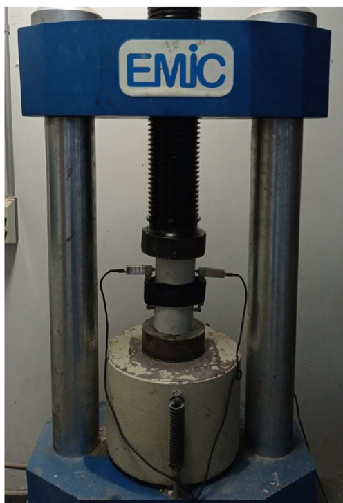
Fig. 5 – Static modulus of elasticity test with the strain gauge detail used.
