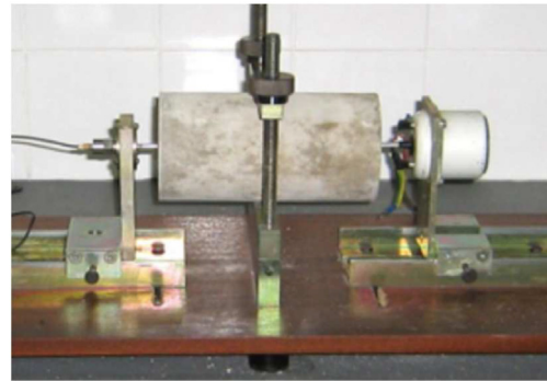
Fig. 6 – Dynamic modulus of elasticity by Resonant Frequency Method.
