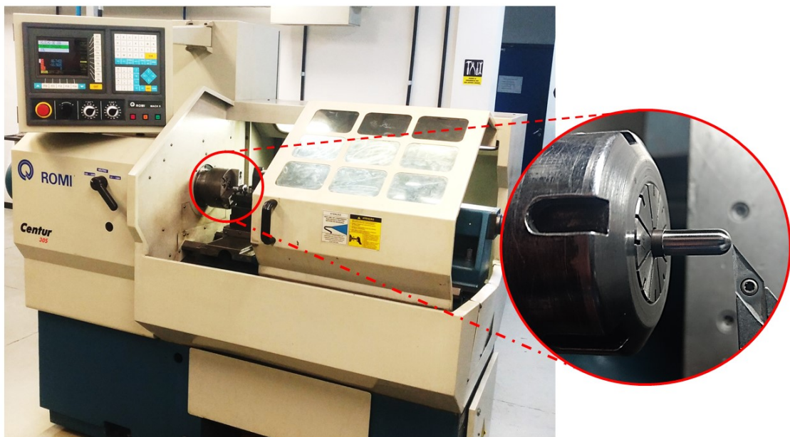
Figura 3.9 – Torno CNC Romi Centur 30S.
