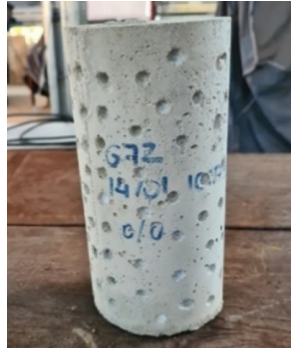
Figure 6. Mechanical chipping surface treatment (holes with drill)
