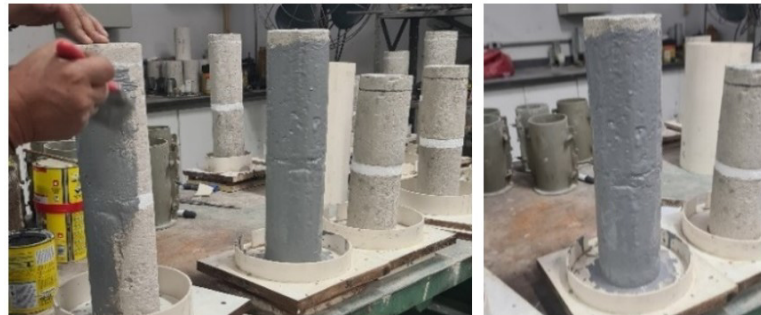
Figure 7. Epoxy adhesive surface treatment
