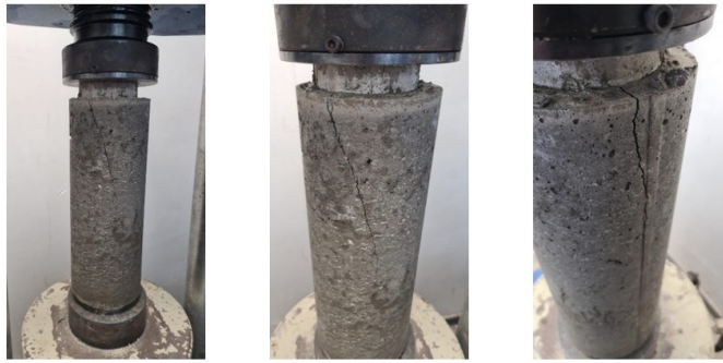
Figure 27. Longitudinal crack in a specimen with t = 2.2\text{cm} / H = 17.5\text{cm}
