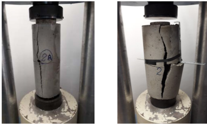
Figure 28. Separation of the core (old concrete) and the jacket (new concrete)
