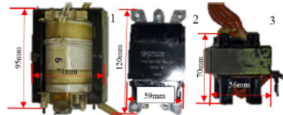
Fig. 5 - 70kHz TSF transformer, 200kHz TSF transformer and 60kHz FB transformer top view
