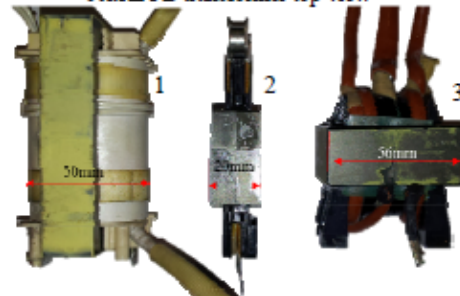
Fig. 6 - 70kHz TSF transformer, 200kHz TSF transformer and 60kHz FB transformer side view
