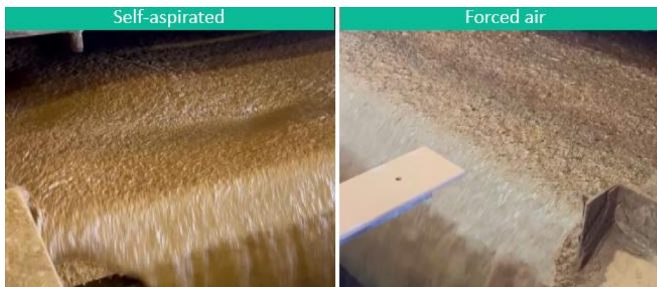
Figure 11.59 - Image of the behavior of the froth surface in the self-aerated and forced-air cell.
