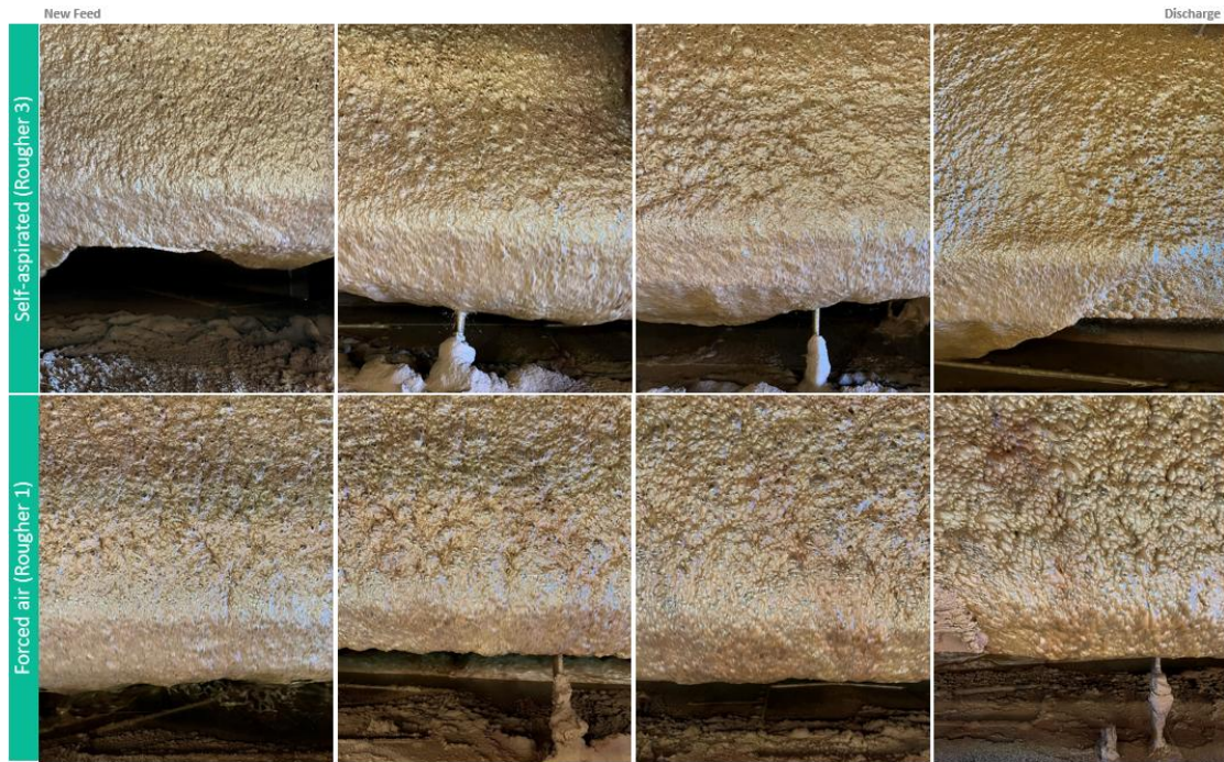
Figure 11.64 - Appearance of bubbles in the overflow on the rougher bench of mechanical flotation.
