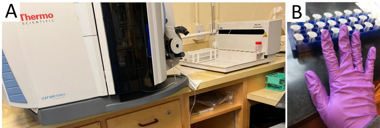
Figure 20 – Equipment utilized to obtain major elements concentration. (A) ICP-OES; (B) clear solution before addition of HNO 3 .
