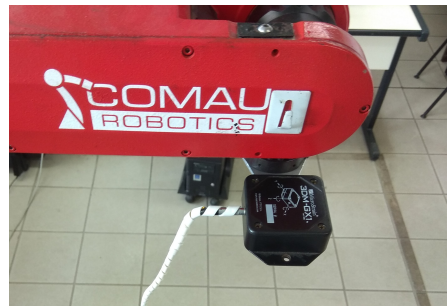
Figure 2. Experimental setup using the MicroStrain 3DM-GX1 ® IMU and the Comau Smart Six ® robot.
