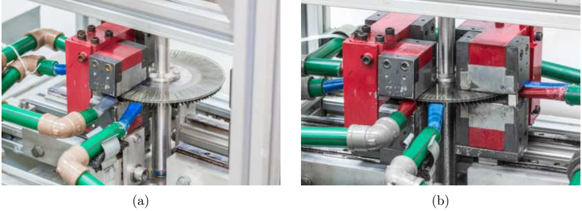
Figure 4.20 – TMM configurations for the performance characterization tests: (a) two-magnetic-volumes configuration (I); (b) four-magnetic-volumes configuration (II).
