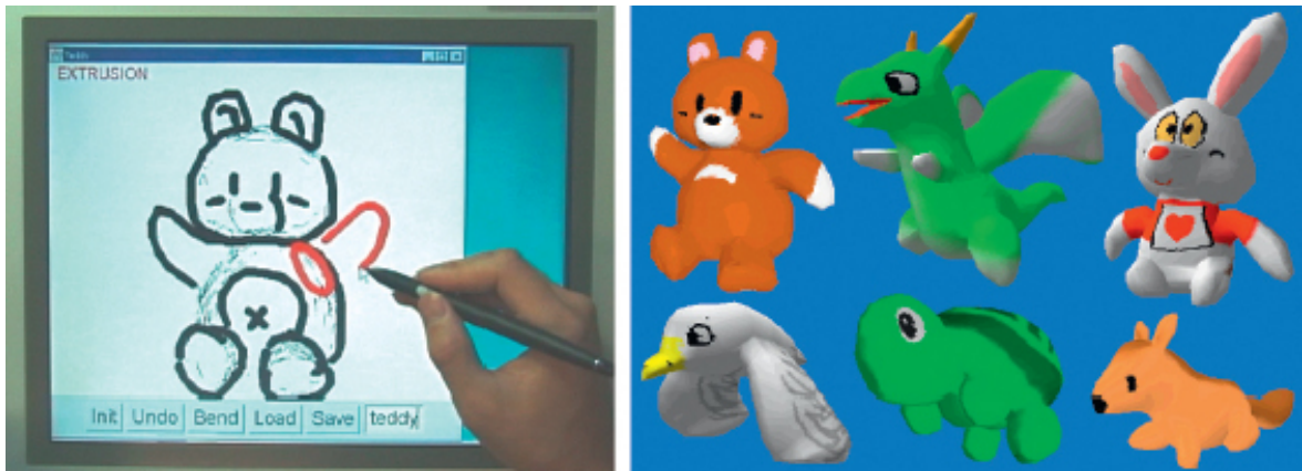
Figure 2.2. An example of Teddy’s user interface and some results achieved by the tool. (Reproduced from [Igarashi et al., 1999])
