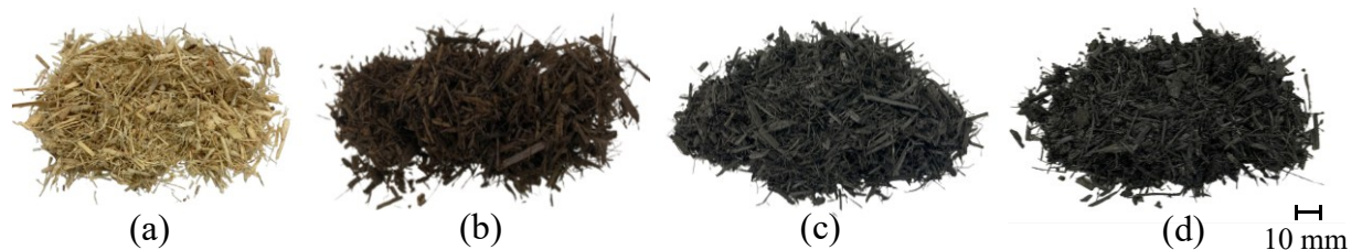
Figure 2.S1. Visual aspect of (a) raw biomass and biochars after pyrolysis treatment at (b) 250 °C, (c) 400 °C, and (d) 550 °C.
