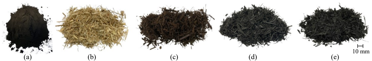
Figure 3.1. Visual aspect of (a) pellet feed, (b) raw biomass and biochars obtained after pyrolysis at (c) 250 ^\circ\text{C} , (d) 400 ^\circ\text{C} , and (e) 550 ^\circ\text{C} .
