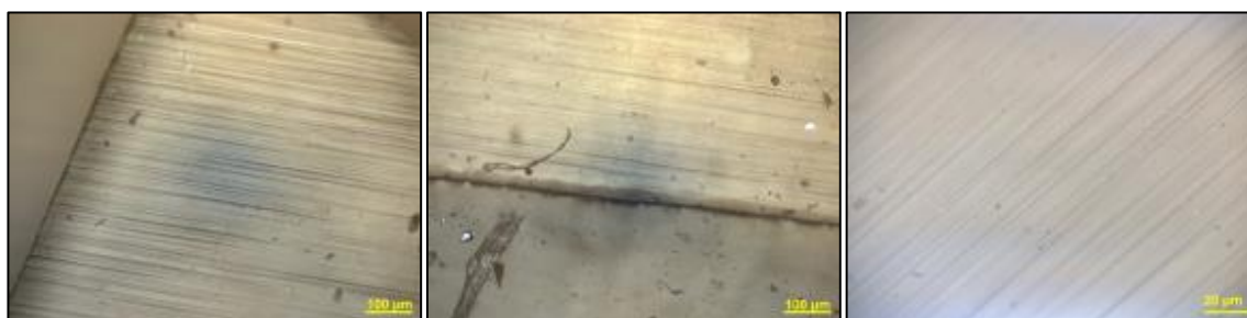
Figure 4 – Optical microscopy of graphene/PDMS composite membrane. Right image: Single layer graphene. Center image: PDMS substrate on the bottom, single layer graphene on the top. Left image: PDMS substrate on the top left border, single layer graphene on the other areas.
