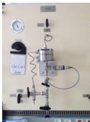
Figure 2 – Apparatus for single gas permeation test.
