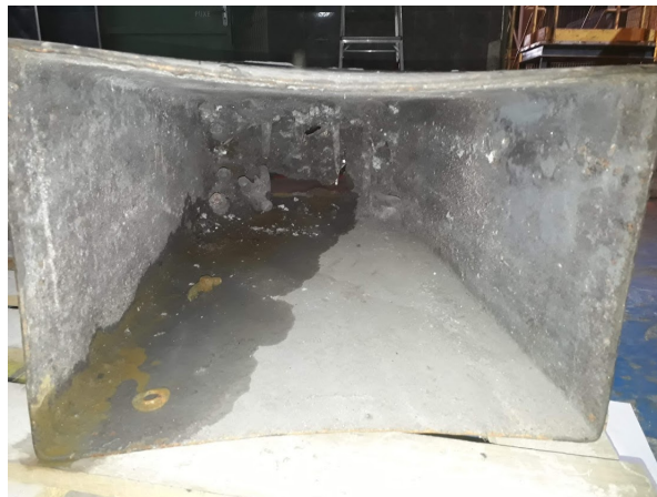
Figure 5.2: Solid shell of a bloom
