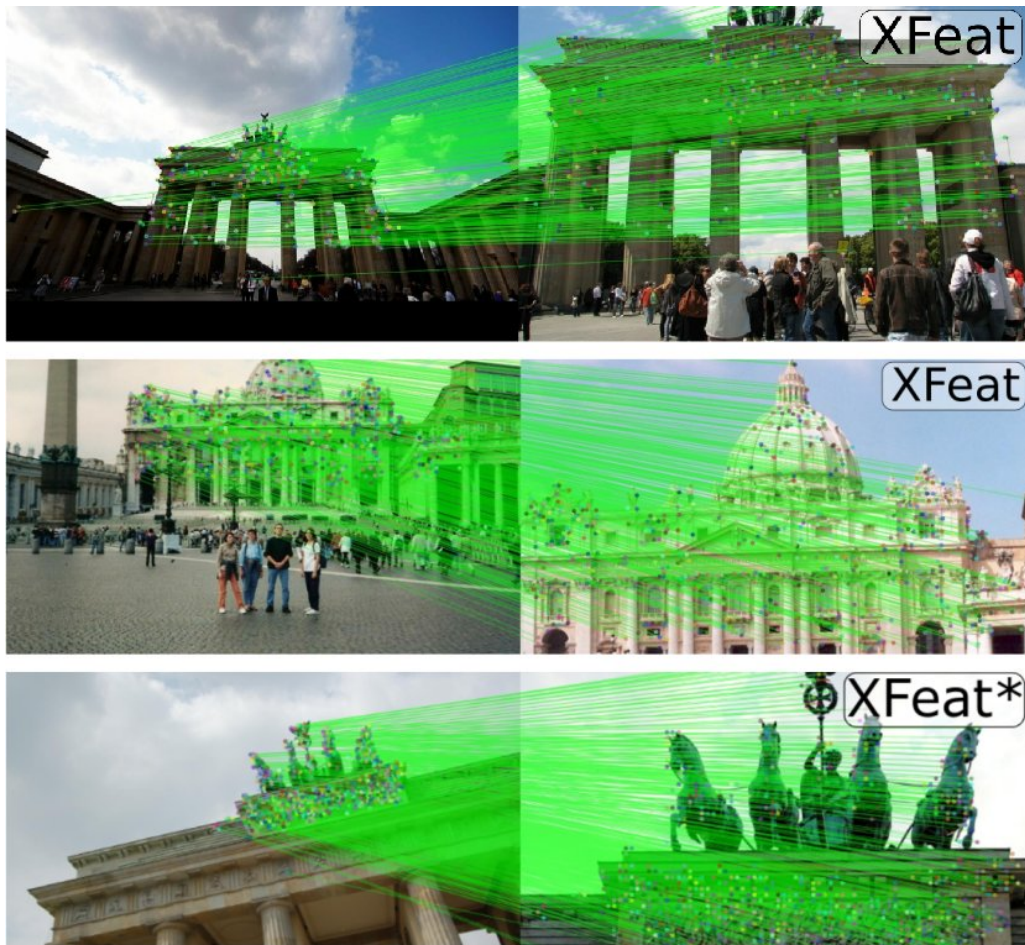
Figure 6.1: Sparse (XFeat) and semi-dense (XFeat*) matching. XFeat stands out with its dual ability to perform both sparse and semi-dense matching, providing fast feature extraction for a wide range of applications from visual localization with sparse matches to pose estimation and 3D reconstruction where denser correspondences deliver additional constraints and a more complete reconstruction.
