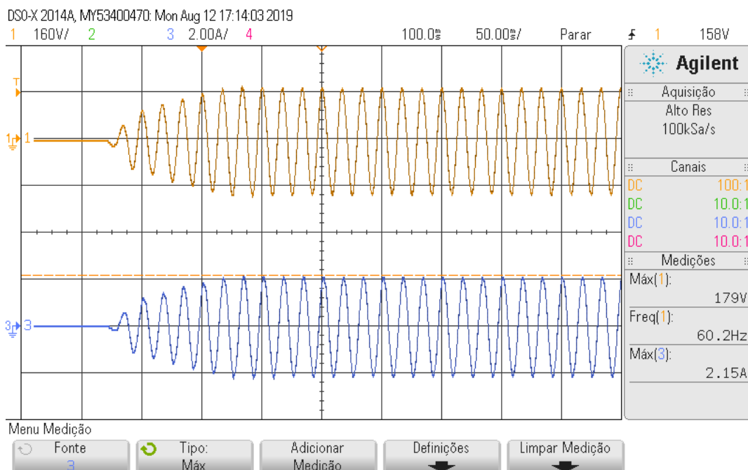
Figure B.8: Droop control implementation in island mode: voltage and output current.
