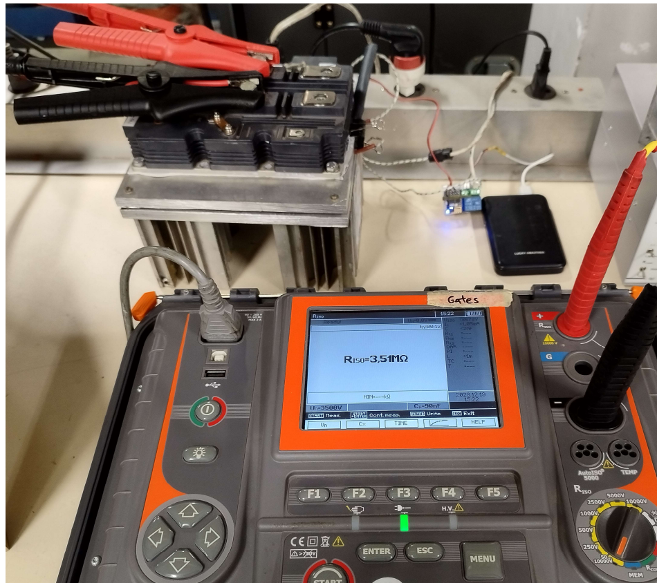
Figure 7.11 Leakage Current Test, Insulation Tester Setup
